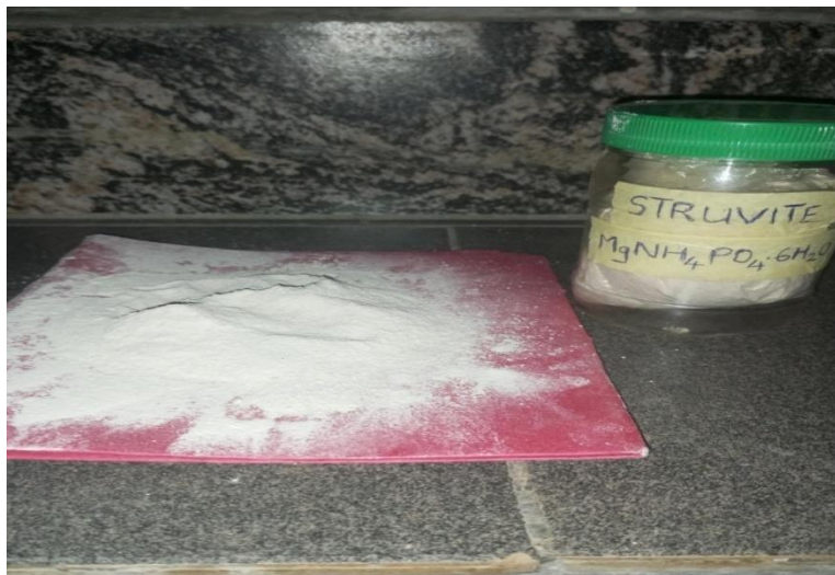
Plate 1: Struvite, recovered from human urin
